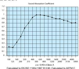
Calculated to EN ISO 11654:1997 ® 0.90, Calculated to ASTM ( 423 - 01- NRC 0.90
